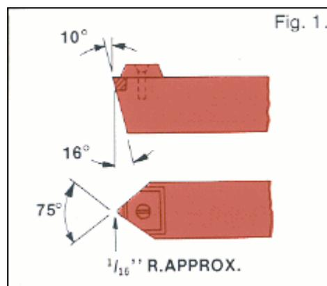
It is possible and practicable to diamond-turn any commutator at full speed. Speeds up to  $45\text{ m/s}$  ( $9000\text{ft/min}$ ) have been handled – providing that the tool rest is rigidly supported in a position that permits a reasonably small overhang of the tool, which must be radially disposed in relation to the
