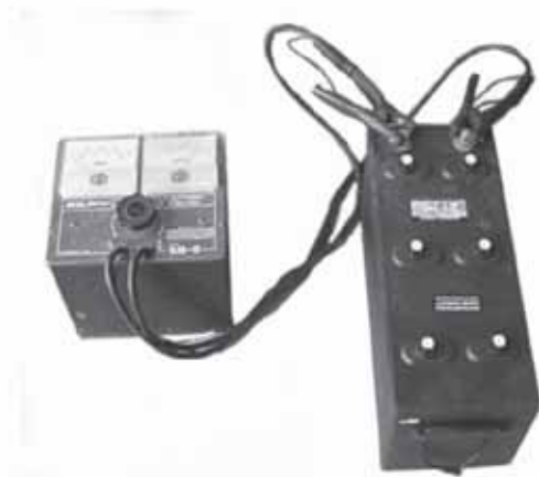
Figure 8: Carbon pile load tester
