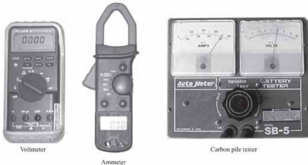
Figure 2: Diagnostic testing equipment.
