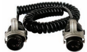
181265 POLYURETHANE ABS COIL. 5-core insulated cable (2 x 4.0 mm 2 . / 3 x 1.5 mm 2 .) 12 V. W/ 2 ABS 5-pin plugs. ISO 7638. Working length 4 mtr. GGVS / ADR approved.
