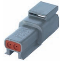
192596 Std pkg 10 A Male holder. Grey. (Terminal: Cargo 192619, secondary lock Cargo 192608).
