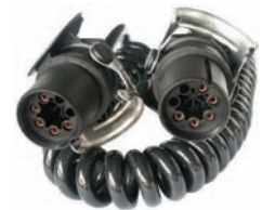
180247 POLYURETHANE ABS COIL. 5-core insulated cable (2 x 4 mm 2 . / 3 x 1.5 mm 2 .) 24 V. W/ 2 ABS 5-pin plugs. DIN 74001, ISO 7638. Working length 4 mtr.
