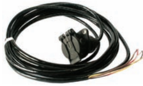
180301 ABS cable assembly w/ socket. 5-core insulated cable - (2 x 4 mm 2 . / 3 x 1.5 mm 2 .) 24 V. W/ 1 ABS 5-pin socket. ISO 7658. w/ 8 mtr. cable.
