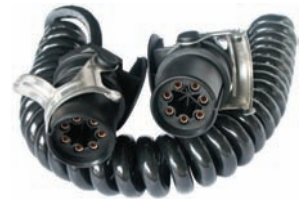
180572 POLYURETHANE EBS COIL. 7-core insulated cable (2 x 4 mm 2 . / 5 x 1.5 mm 2 .) 24 V. W/ 2 EBS 7-pin plugs. DIN 74001, ISO 7638. Working length 4 mtr.
