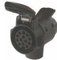
181461 7-pin plug to 13-pin coupling socket. W/o cable. Connect pos. 2/54 g on 7-pin to pos. 9 and 10 on 13-pin. (Continuous power supply). And connect 3/31 on 7-pin to pos. 3, 11 and 13 on 13-pin.
