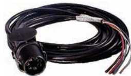
180304 ABS cable assembly w/ plug. 5-core insulated cable (3 x 1.5 mm 2 . / 2 x 4 mm 2 .) 24 V. W/ 1 ABS 5-pin plug. ISO 7658. W/ 10 mtr. cable.
