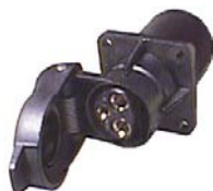
180306 Socket, plastic. 4 hole fixing flange. Flat tonque terminals. Rated at 1x5, 2x25 Amp. 12 V. continuous use.
