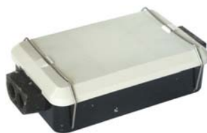
Plastic, sealed against dust and water. W/ 4 cable entries. W/ locking clamps. Dim.: 120 x 79 x 36 mm.
