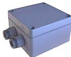
Plastic, sealed against dust and water. 6 x 8 terminals flat-plug connection. W/ locking screw. Dim.: 105 x 105 x 64 mm.
