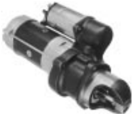
CM8016 Ref No: CM-8016 24 Volt, CW, 10 Tooth Used On: Mack Truck, Consolidated Diesel Wet Clutch
